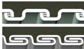
Square-Locked Design with cord packing 3/8" - 1-1/4"
