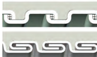
Square-Locked Design with cord packing 5/16" - 1-1/4"
