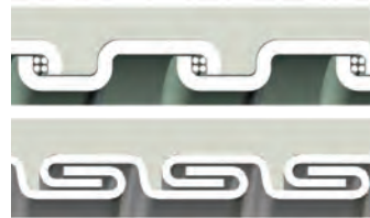
Square-Locked Design with cord packing 3/8" - 1-1/4"
